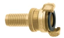
The GEKA® plus SH suction and high-pressure coupling is an ideal solution for all hose lines. It is secured against becoming loose and completely sealed when in a non-pressurised state thanks to safety nubs and screw rings.
